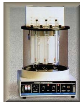
Figure 5. Zietfuchs Cross-Arm Viscometer
