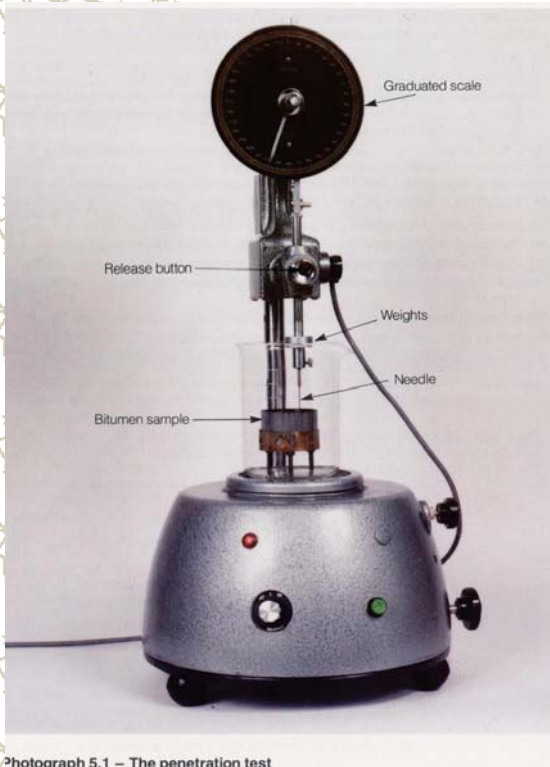
Photograph 5.1 – The penetration test
