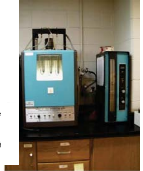
Figure 4. Asphalt Institute Vacuum Viscometer
